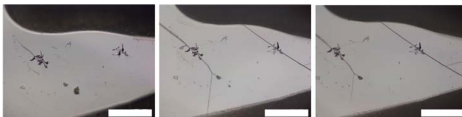
Figure 5. Optical micrographs of the same portion of a p-WSe 2 crystal surface before stability testing (left), after testing under acidic conditions (center), and after testing under alkaline conditions (right). Scale bars are 0.2 mm.
